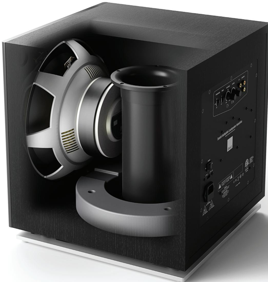
*Any risk of port noise derived from the down-firing bass vent itself is seriously reduced by its convex tapered design. The vent has undergone extensive testing, measuring and listening when it comes to dimensions and placement, in order to optimize interaction with the cabinet and woofer.*
