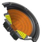
The cone and dust cap can move very fast, because it is made of a mixture of paper pulp and wooden fibres (a very light composite). The composite is rather stiff, which to some extent will cause break-ups of the cone at certain frequencies. These break-ups are eliminated by using a coating on the cone.
