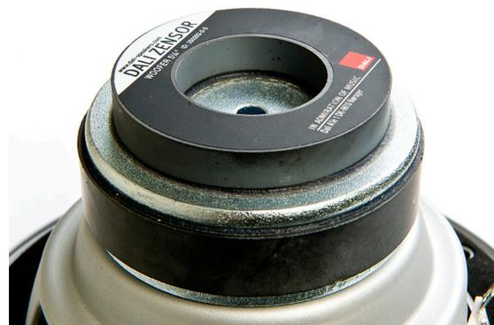
On the ZENSOR 1 the need for a high B/L-product was especially important in order to maintain superior control of the woofer in this limited cabinet volume. Therefore an extra magnet has been added to the motor of the ZENSOR 1 woofer.
