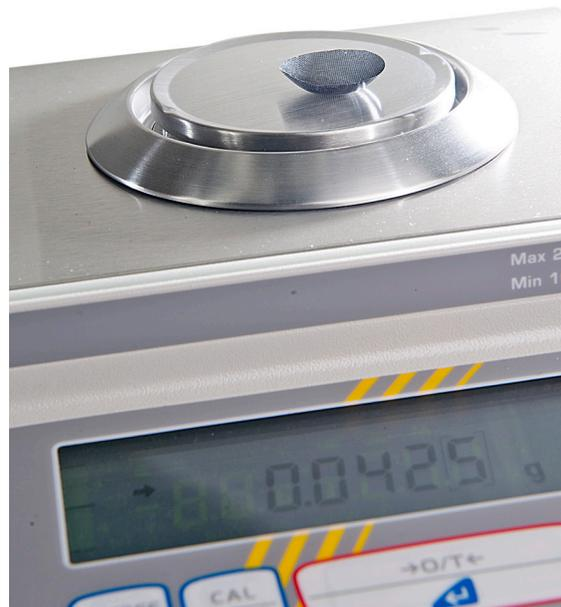
*The ZENSOR tweeter is constructed on the basis of an ultra light-weight weave fabric. Compared to most soft dome tweeters in the market the DALI dome material is less than half the weight; 0.056 mg per mm<sup>2</sup>.*
