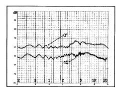
Frequency response on axis and  $45^{\circ}$  off axis.
